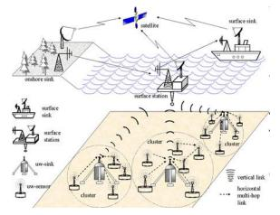
In this module we create a UNS, It consists of a number of underwater sensor nodes, underwater sink, surface station, Autonomous Underwater Vehicles (AUVs) that are deployed to perform collaborative monitoring and resource exploration tasks over a given area.
